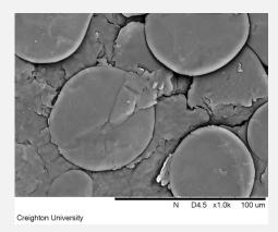
Lucitone wear facet above is uniform and smooth. Aged acrylics however, after momoner leaching would likely exhibit brittle fracture. The higher magnification shows the acrylic polymer bead surrounded by the continuous phase monomer gel.
