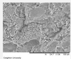
The KeySplint Soft wear facet appears slightly distorted and is suggestive of the occurrence of some plastic deformation initiated by the wear antagonist force or possibly temperature rise at the wear surface. No clear evidence of cracking is noted in the higher magnification image.
