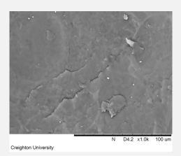
The morphology of the standard clear disc is similar to the Lucitone. The higher magnification image does suggest the beginning of some surface and sub-surface cracking.
