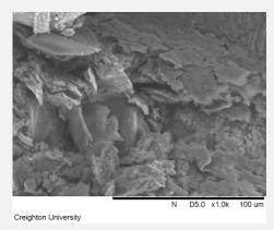
The wear facet above is distorted and in conjunction with the higher magnification image is suggestive of brittle fracture.
