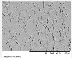
The KeySplint Hard surface in smooth without evidence of cracking or crazing. The pattern is suggestive of excellent abrasion resistance.
