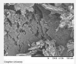
The dual laminate facet and higher magnification image show evidence of surface and sub-surface cracking. The facet is highly irregular but does not exhibit the swirling deformation pattern seen with other materials. The ragged edge in the wear facet is suggestive of edge fracture of the material.
