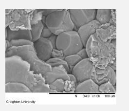
Resembling the force or temperature plastic deformation of the KeySplint Soft above material the KeySplint Soft Clear for Carbon material's wear facet shows some clear evidence of swirling consistent with the 30 degree rotation of the wear antagonist. Based on the dynamic modulus change with temperature this finding is likely due to an increase in temperature at the contact point. The higher magnification does not show any cracking.
