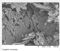
The dual laminate facet and higher magnification image show evidence of surface and sub-surface cracking. The facet is highly irregular but does not exhibit the swirling deformation pattern seen with other materials. The ragged edge in the wear facet is suggestive of edge fracture of the material.
