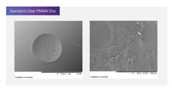
The morphology of the standard clear disc is similar to the Lucitone. The higher magnification image does suggest the beginning of some surface and sub-surface cracking.
