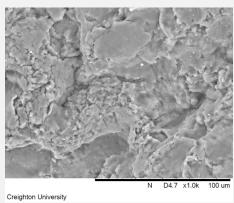
The KeySplint Soft material's wear facet shows some clear evidence of swirling consistent with the 30 degree rotation of the wear antagonist. Based on the dynamic modulus change with temperature this finding is likely due to an increase in temperature at the contact point. The higher magnification does not show any cracking.
