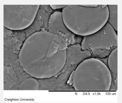
Lucitone wear facet above is uniform and smooth. Aged acrylics however, after monomer leaching would likely exhibit brittle fracture. The higher magnification shows the acrylic polymer bead surrounded by the continuous phase monomer gel.
